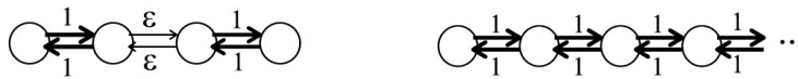
Figure 1: Nearly completely decomposable Markov chain (left), one-dimensional Markov chain with identical transition rates (right)
